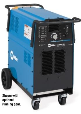
Compact design occupies minimal space with a footprint of 3.3 sq ft (.30 m<sup>2</sup>) and total weight of 165 lb (74.9 kg). The power source can be conveniently mounted in almost any location and the open base allows for easy lift truck access for portability.
