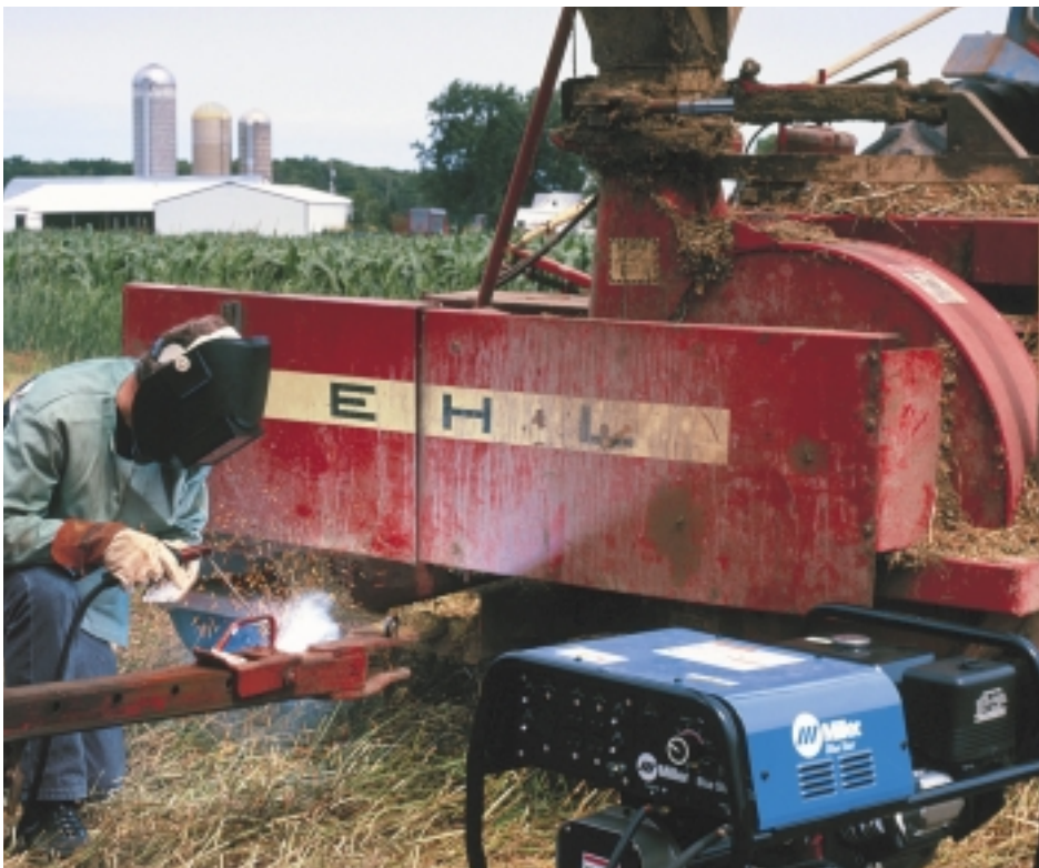
For the fastest field repair possible, this farmer brought a lightweight welding generator directly to the broken implement. After a quick Stick weld on the hitch, he resumed work.
