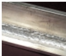
Unretouched photo of pulsed MIG weld bead
